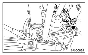
(1) Brake caliper assembly
