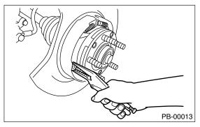
7) Remove the strut and strut spring.
